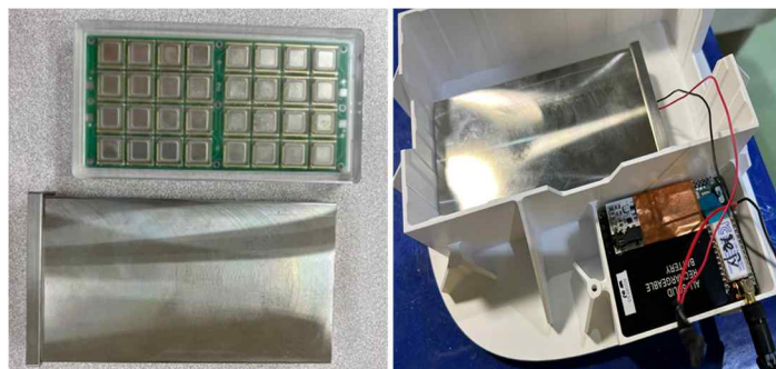
Figure 1. Prototype of Ni-63 betavoltaic battery and application of sensor system to measure spatial radiation.
