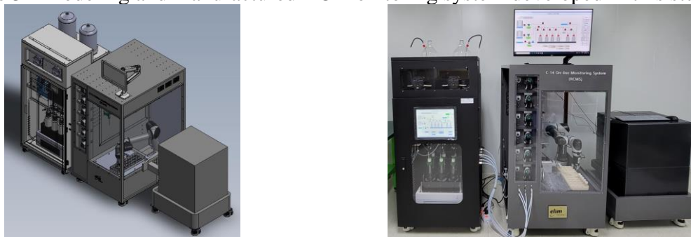
Figure 1. 3D modeling and manufactured fully automated ^{14}\text{C} monitoring system.
